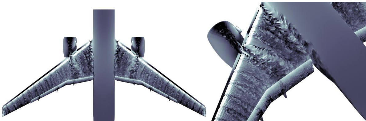
Figure 4: Flow structures over the surfaces of CRM-HL Case 2.4 (760M DoF)
